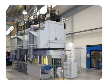
The drying area has three 100 kg capacity ST100 dryers and the ironing area consists of two ironing systems. One, designed for large flat items of linen such as sheets and bedspreads, is equipped with an automatic 3-station DRF feeder, a PC120 Gas flatwork ironer with two rollers and an FL folder. The other, designed for small flat articles of linen such as pillowcases, has an automatic 2 position DRB feeder, one single-roller PC120 Gas flatwork ironer and an FL Folder.
